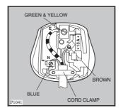
The wire coloured green and yellow must be connected to the terminal marked with the letter «E» or by the earth symbol  $\stackrel{\bot}{=}$  or coloured green and yellow.
